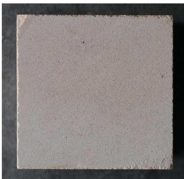
Figure 1: Image of hand specimen, width of sample is 50 mm
